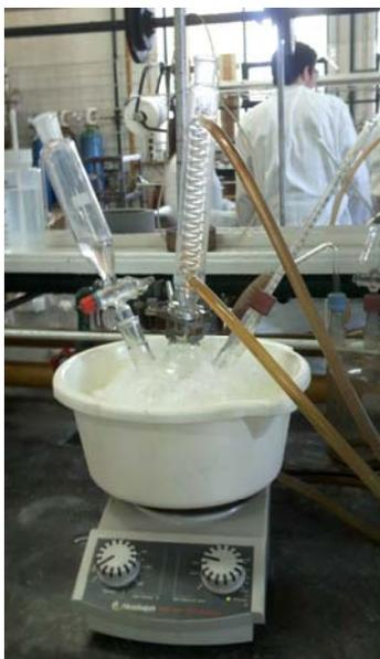
**Figure SM 5.2.1.1** – Reaction set apparatus for 1,4-di-*t*-butyl-2,5-dimethoxybenzene
