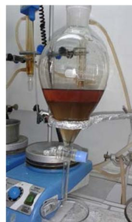
Liquid-liquid extraction. From left to right: first extraction, second extraction and organic layers wash with water.
