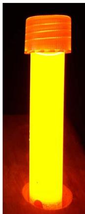
**Figure SM 5.2.9.6** – Chemiluminescence reaction using bis(2,4,6-trichlorophenyl oxalate).
