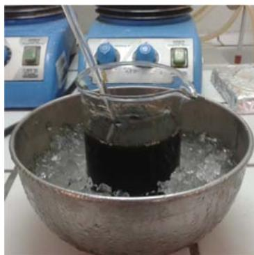
Reaction mixture in an ice bath after neutralization
