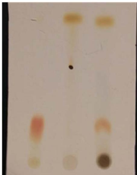
**Figure SM 5.2.5.4** Thin-layer chromatography. ZnTPP(left), TPP (center), and crude reaction mixture (right). Eluent hexanes:CH<sub>2</sub>Cl<sub>2</sub> (2:1 v/v)
