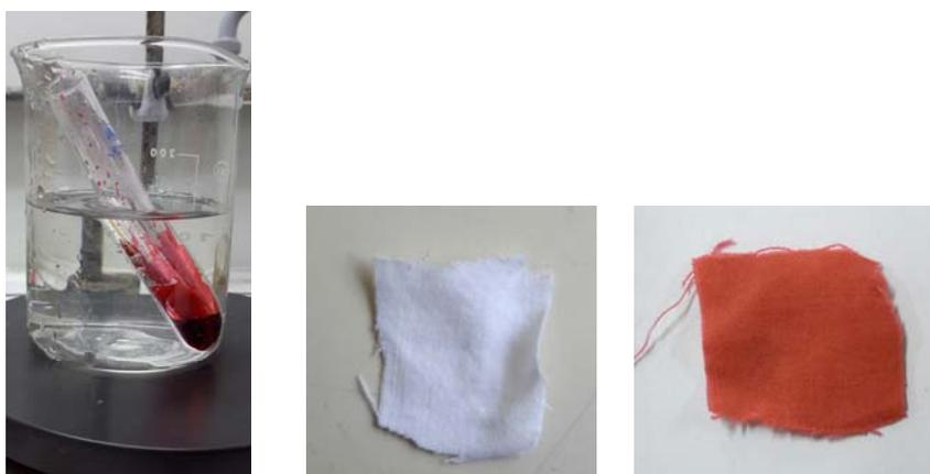
**Figure SM 5.2.9.5** – Dyeing process of a piece of cotton with eosin
