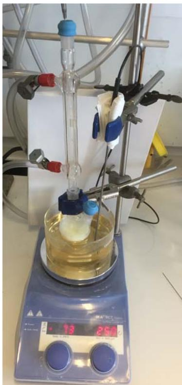
**Figure SM 5.2.11.6** - Picture of the reaction mixture after reflux for three hours. The color of the reaction mixture changes to pale yellow.
