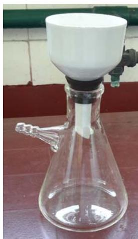
**Figure SM 5.2.1.2** – Vacuum filtration set-up.
