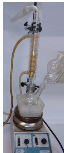
Figure SM 5.2.8.1 Left - Photo of the apparatus for heating at reflux in dry conditions (Laboratory session 2); Right - Photo of the apparatus for the Friedel-Crafts acylation of thiophene (Laboratory session 4).
