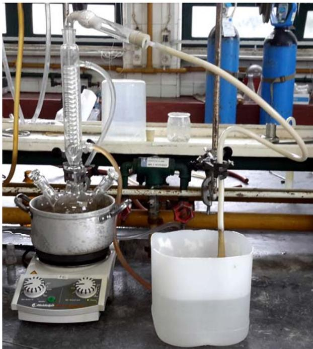
**Figure SM 5.2.2.1** – Reaction set-up apparatus for 4,4'-di-tert-butylbiphenyl
