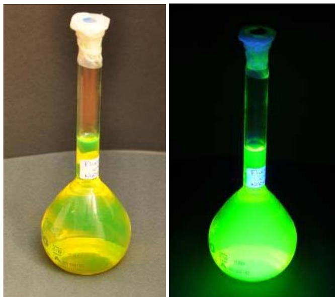
**Figure SM 5.2.9.1** - Fluorescein basic solution under sun light and UV light
