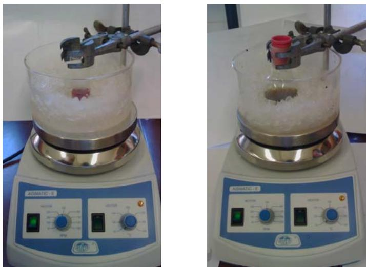
Figure SM 5.2.14.1 Left - Photo of the apparatus for the preparation of the diazonium salt (laboratory session 5i); Right - Photo of the apparatus for the coupling of the diazonium salt with the thienylpyrrole derivative (laboratory session 5ii).
